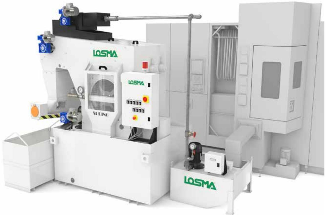
Self-cleaning systems from Spring series are suitable for many machine tool types, such as: machining centers, deep drilling, transfer, grinding and milling machines, machining with special tools requiring high-pressure coolant.
